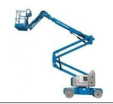
**Articulating Boom Aerial Lift** This aerial lift has at least 2 hinged sections which are used to increase mobility.
