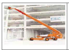
**Extendable / Telescoping Aerial Lift** This aerial lift has a boom that extends horizontally and vertically.
