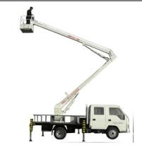
**Vehicle Mounted Aerial Lift / Bucket Truck** The lift platform is an integral part of an over the road vehicle.
