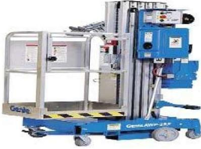
A blue man lift with a platform that is raised vertically, allowing workers to reach heights without moving horizontally.                                  | <b>Man Lift / Cherry Picker</b> This piece of equipment lifts personnel vertically, but not horizontally.                 |
