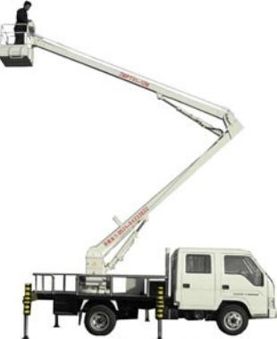
A white aerial lift truck with a long, articulated boom extending upwards and to the left. A worker is standing on the lift platform at the end of the boom. | <b>Vehicle Mounted Aerial Lift / Bucket Truck</b> The lift platform is an integral part of an over the road vehicle.      |
