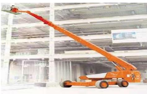
**Extendable / Telescoping Aerial Lift** This aerial lift has a boom that extends horizontally and vertically.
