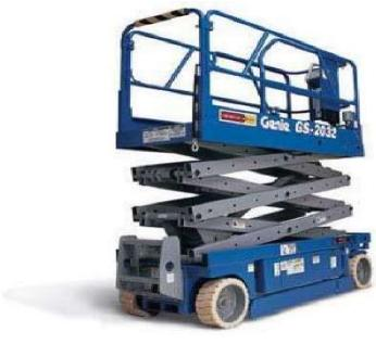
A blue scissor lift with a platform that is raised vertically, allowing workers to reach heights without moving horizontally.                              | <b>Scissor Lift</b> This piece of equipment lifts personnel vertically, but not horizontally                              |
